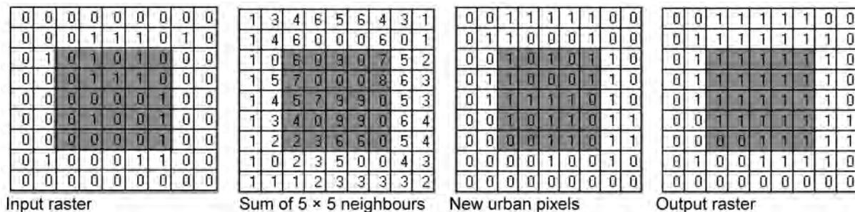
**Figure 3** The concept of CA model to simulate the future urban pattern
