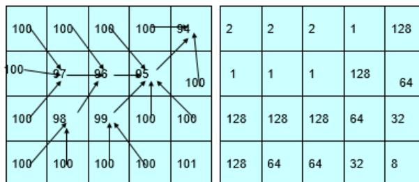
**Figure 6** Flow direction grid (right) has been generated from the DEM (left)
