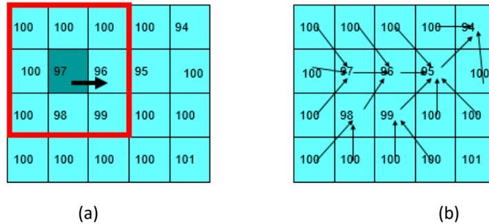
**Figure 4** (a) Moving window search to find out the lowest surrounding pixel value, (b) A grid shows water flow for all of the pixels in the grid
